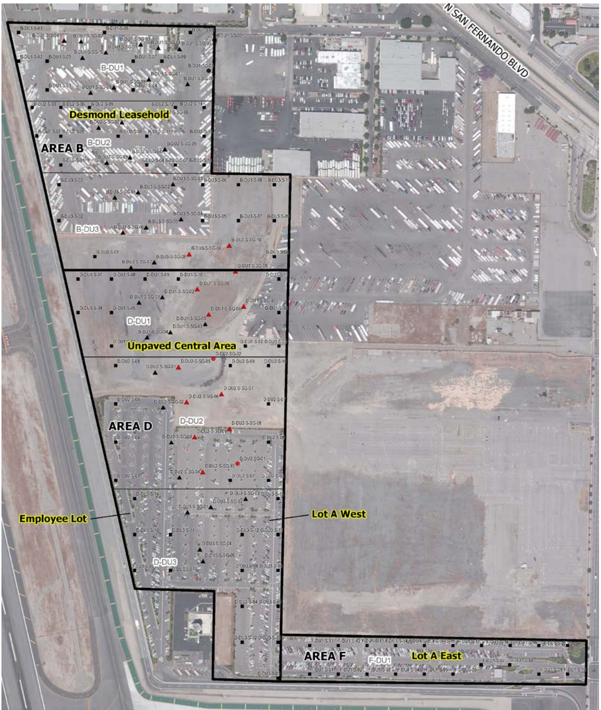
EFI Global analyzed 74 soil samples and 137 soil vapor samples from a variety of locations across four principal areas: the Desmond Leasehold, the Unpaved Central Area, the Employee Lot/Lot A West and Lot A East.
