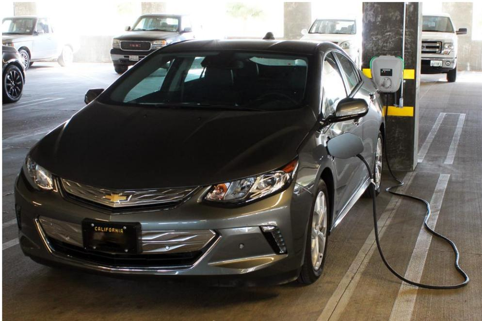
*An electric vehicle charges, using one of the Siemens VersiCharge Level 2 Plug-In Electric Vehicle (PEV) charging stations in the Hollywood Burbank Airport's Valet parking garage. The charging stations were installed by the Burbank Water and Power Department (BWP).*
